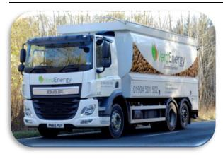
VerdEnergy only supply ENplus A1 wood pellets, delivered using specialist pneumatic, earth bonded lorries, smooth bore low friction hoses, which are only used for wood pellet deliveries to limit contamination issues.
